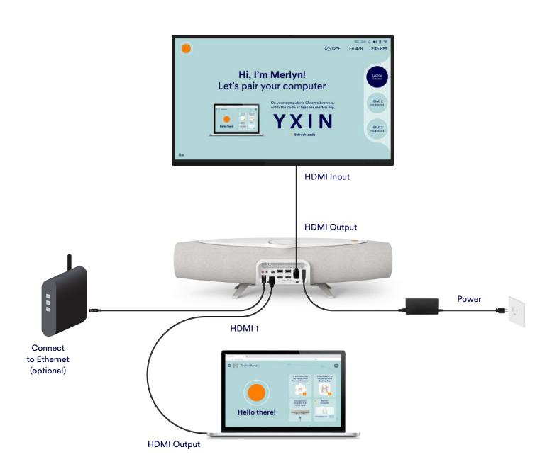
2. How to connect a Smart Board with touch capabilities
